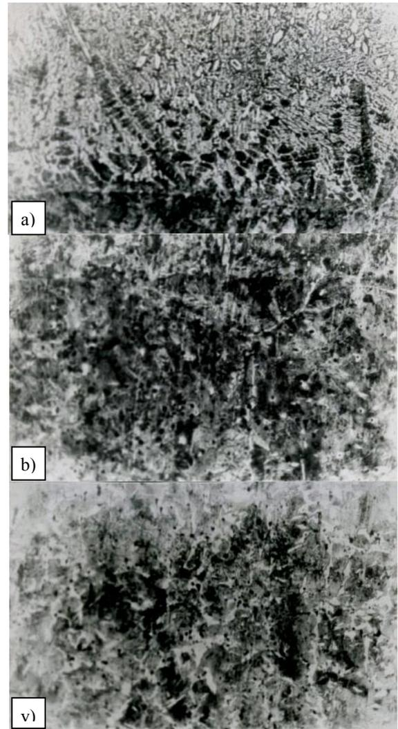
**Fig. 1.** The microstructure of hard-alloyed coating obtained by casting parts from steel 35GL on gasified models: *a*-hard-alloyed coating with the transition to high carbon sublayer; *b*-hypereutectoid structure of the sublayer; *v*-the base metal.
