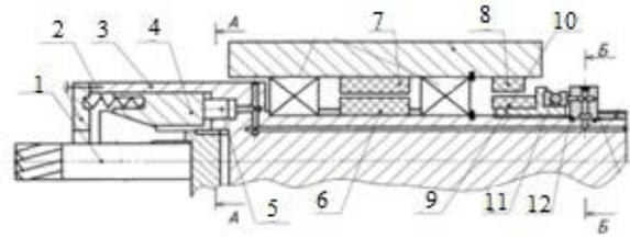
Figure 6 - Longitudinal section of the spindle-motor assembly, containing the main motion drive, helical gear and collet chuck
