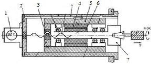
Figure 4 - Longitudinal section of the spindle-motor assembly
