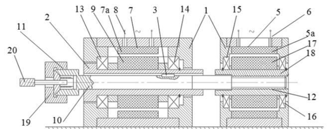
Figure 7 - Longitudinal section of the spindle-motor assembly
