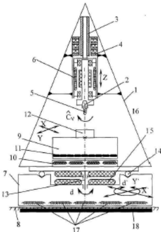
Figure 8 - Pyramidal arrangement of the machine tool without mechanical transmission
