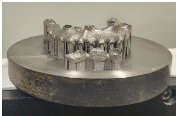
Fig. 9. Frameworks for metal-ceramic dentures, manufactured of Ti6Al4V alloy by selective laser melting
