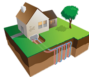
Fig. 3. Vertical ground heat exchanger [6]
