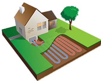
Fig. 2. Horizontal ground heat exchanger [6]
