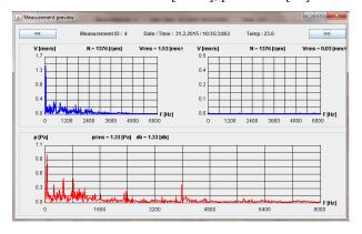
Fig. 7. Spectra and measured values on undamagedbearing when the shaft is aligned at 1376 rpm - acceptablecondition
