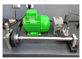
Fig. 2. Appearance of the bearing test rig
