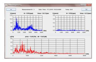
Fig. 6. Spectra and measured values on badly damaged bearing when the shaft is aligned at 1378 rpm- unacceptable condition
