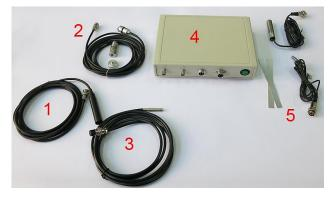
Fig. 4. VibroLog device with sensors
