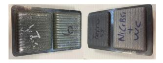
Fig. 3. Samples coated by laser cladding method
