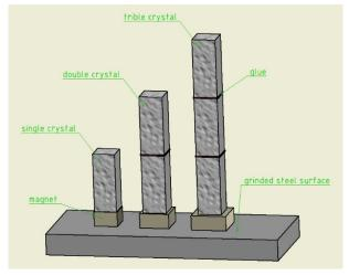
Fig. 5. Test specimens: single crystal, double crystals, and triple crystals
