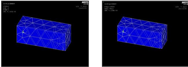
Fig. 15. Longitudinal (x-direction) and transverse deflection (z-direction) analysis of single PZT crystal test specimen at resonance frequency and 220 V Voltage
