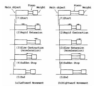
Fig. 2. IDM based mechanism movement principle [2].
