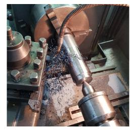
*Fig. 1. Experimental setup (minor cutting edge angle of*  $k_1 = 25^{\circ}$  *is achieved by rotating the tool post)*
