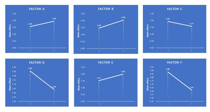
Fig. 2. Main effects plots of turning parameters on surface roughness
