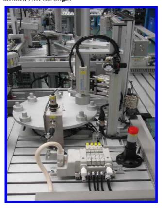
Fig. 5. Manipulators of the cover classification module
