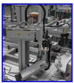
Fig. 6. Cover rejecting and transferring module
