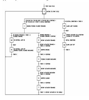
Fig. 8. Program for the feeding module
