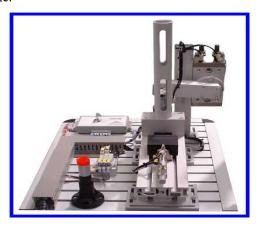
Fig. 3. Manipulators of the feeding module
