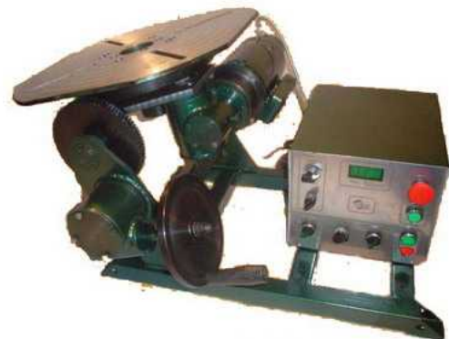
Fig. 1. Universal rotary welding device [14]
