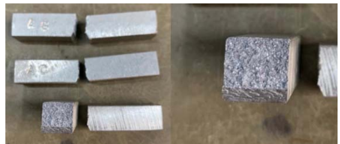
Fig. 7. Crack propagation in Charpy V-notch specimens
