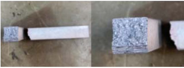
Fig. 9. Crack propagation in Izod V-notch specimens
