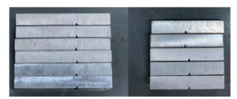
Fig. 4. Charpy and Izod test specimens
