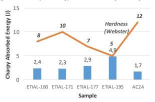
Fig. 6. Relation between absorbed impact energy and hardness
