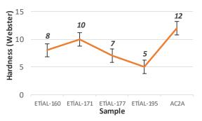
Fig. 5. Hardness of the Charpy and Izod notch impact test specimens
