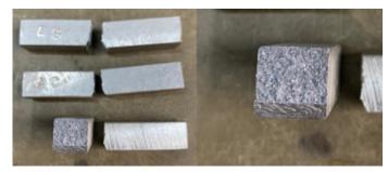
Fig. 7. Crack propagation in Charpy V-notch specimens
