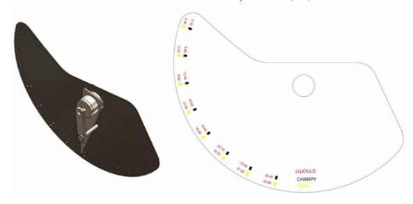
Fig. 2. Charpy & Izod impact energy indicator (J)
