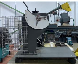
Fig. 1. Designed Charpy & Izod impact tester
