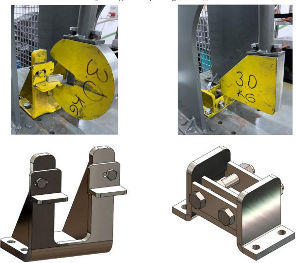
Fig. 3. Charpy and Izod specimen clamps
