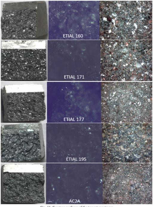
Fig. 11. Fracture surfaces of the impact specimens
