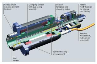
Fig. 2. Typical structure of SIEMENS motor-spindles
