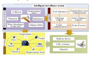
Fig. 3. System architecture and work processes of intelligent spindles
