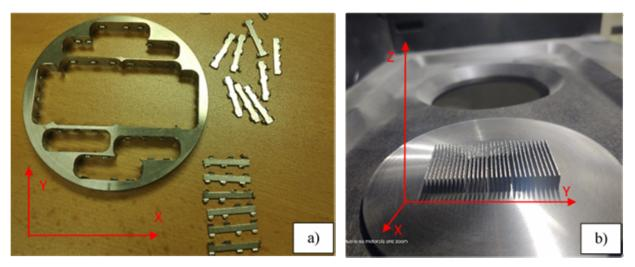
Fig. 1. Ti6Al4V alloy disc with milled samples -a) and disposition of the samples on the working table of SLM machine -b)
