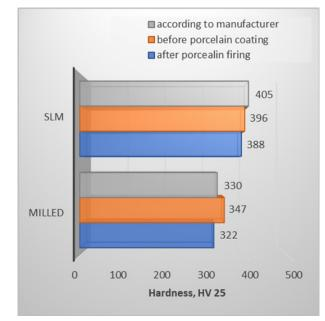
Fig. 4. Micro-hardness of Ti6Al4V alloy
