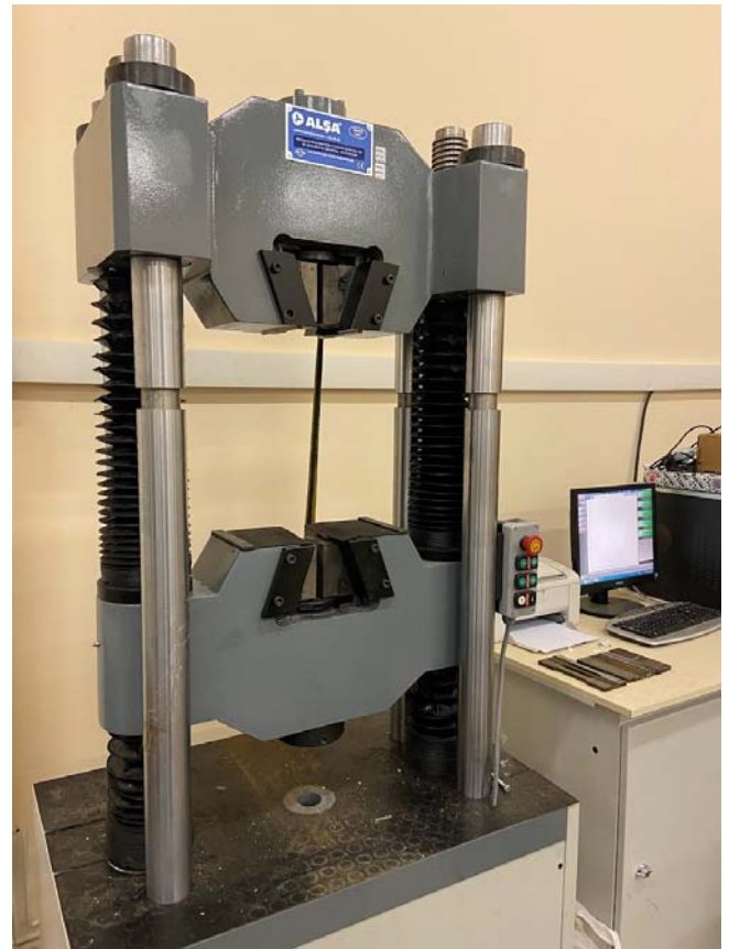
Fig. 5. Tensile testing device (ALŞA AB-0066-K)
