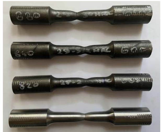
Fig. 7. Fractured tensile specimens after tensile testing
