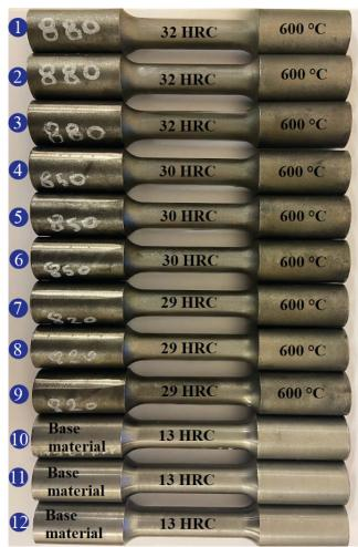
Fig. 3. AISI 4140 tensile test specimens after heat-treatment
