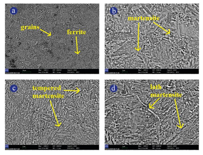
Fig. 9. FESEM microstructure of AISI 4140 a) Base material (1.00KX magnification) b) Heat-treated at 820 °C (3.00KX magnification) c) Heat-treated at 850 °C (2.00KX magnification) d) Heat-treated at 880 °C (3.00KX magnification)
