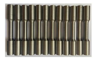
Fig. 2. AISI 4140 tensile test specimens
