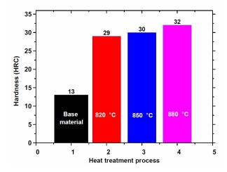
Fig. 6. Rockwell-C hardness graph
