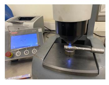
Fig. 4. Rockwell-C hardness measurement
