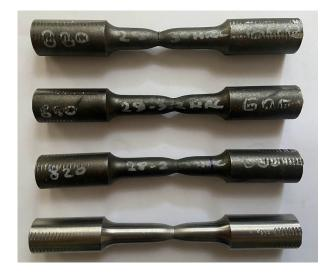
Fig. 7. Fractured tensile specimens after tensile testing
