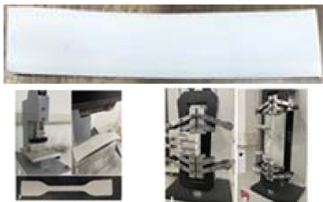
Fig. 7. Strip sampling and tensile testing of samples
