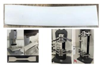
Fig. 7. Strip sampling and tensile testing of samples
