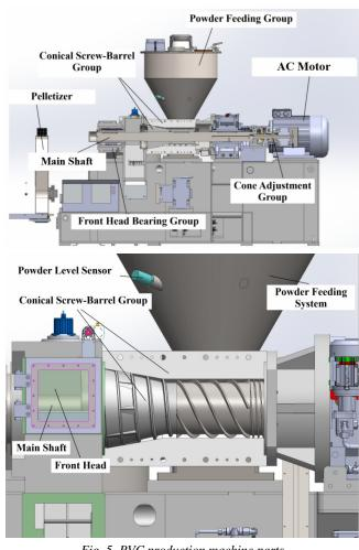
Fig. 5. PVC production machine parts
