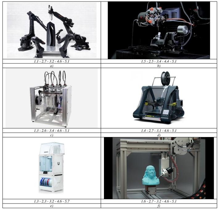
Fig. 4. Commercially available hybrid 3D printers and their morphological formulas: a - AI Build, b - Diabase Engineering H-Series, c - E3D ToolChanger, d - Zmorph Fab,e - Ultimaker S5 Bunlde, f - 5Axis Maker
