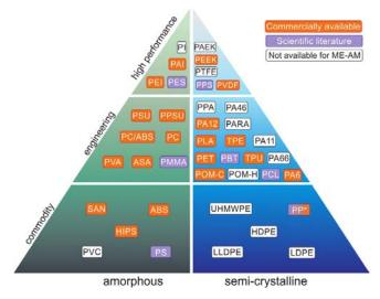
Fig. 2. Groups of materials for FFF 3D-printing technology
