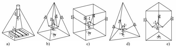
Fig. 5. Layouts of small-sized machine tools obtained by the method of multilevel morphological analysis [6]
