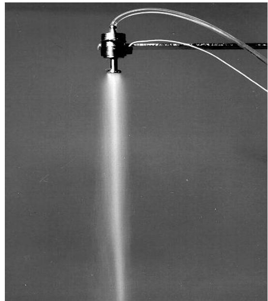
Fig. 1. Narrow, dense aerosol plume during ultrasonic atomization
