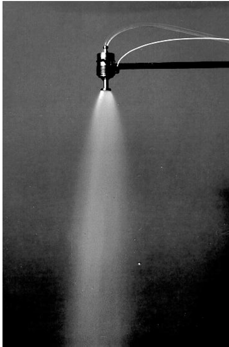
Fig. 2. Extended aerosol plume during ultrasonic atomization
