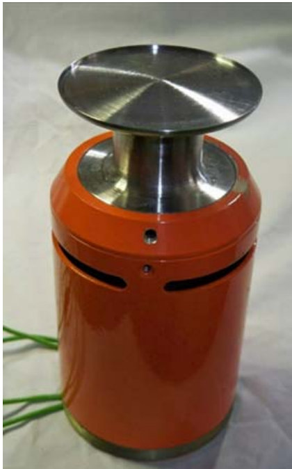
Fig. 8. High performance ultrasonic dispersant with applied axial excitation oscillations in the nodal area of the atomisation surface bending oscillations
