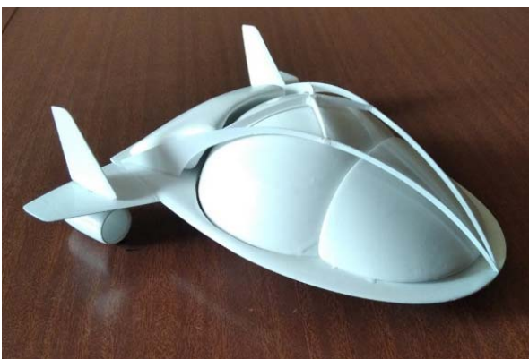
Fig. 4. Hybrid aircraft concept: 1 - light gas balloon, 2 - gondola, 3 - keel, 4 - height rudder, 5 - engine, 6 - stiffeners, 7 - rigid frame
