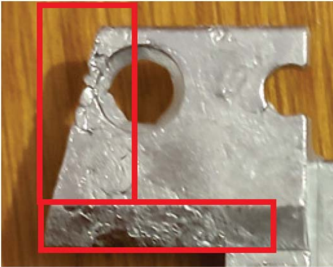
Test sample 3 0.8-1.1 ml/lubricated sample (left side, top surface)
