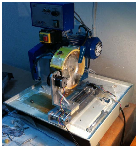
Fig. 6. The machine of the SKU model of Avalon firm (Poland), equipped with the model prefix of automatic radial giving of balls
