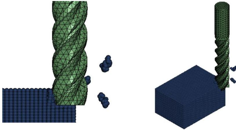
Fig. 10. Formation chip from milling simulation
