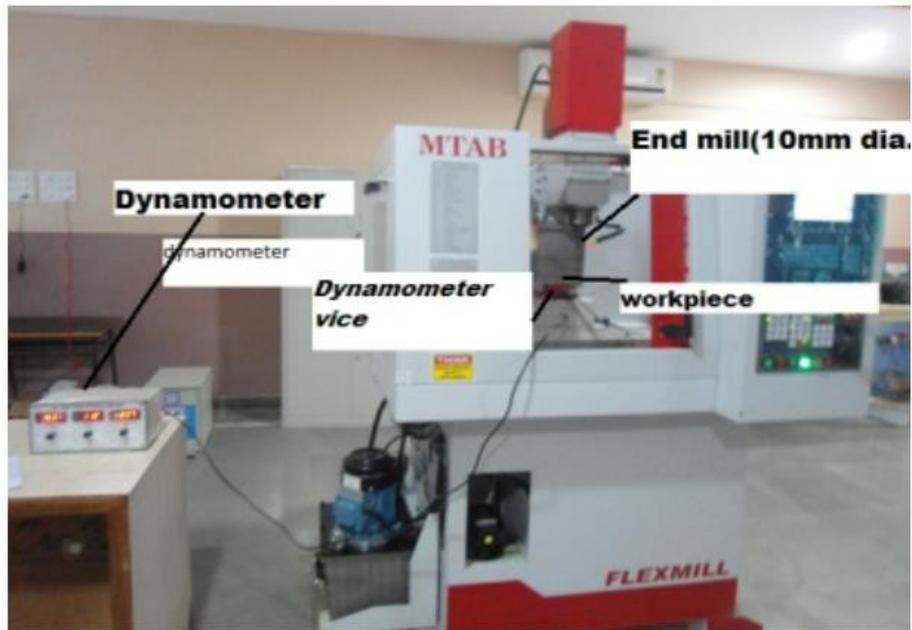
Fig. 4. Experimental milling setup [41]
