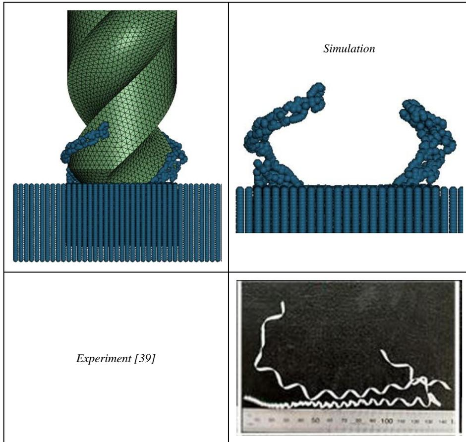
Fig. 9. Formation chip from simulation and experimental
