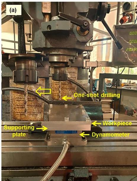
Fig. 3. Experimental setup [39]
