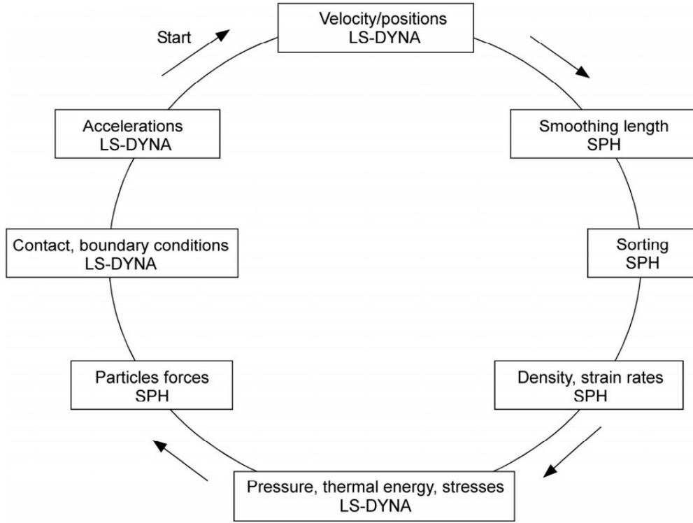
Fig. 2. The time integration loop in LS-DYNA
