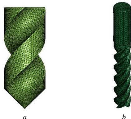
Fig. 6. Finite element of drilling tool (a) and milling tool (b)
