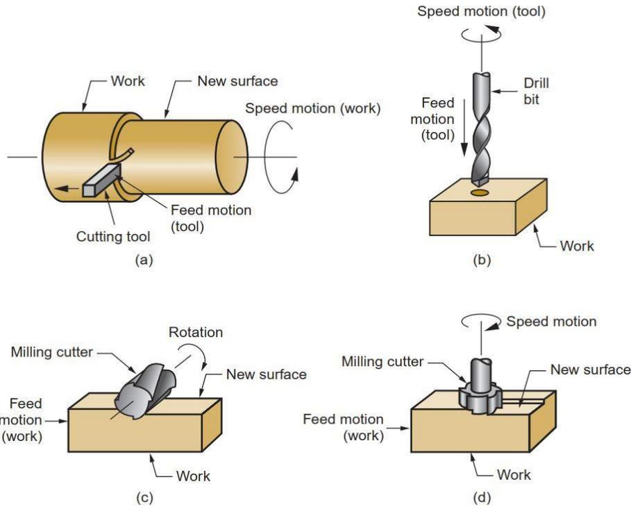
Fig. 1. Three most common types of machining processes: (a) turning, (b) drilling, and (c), (d): two forms of milling [36]
