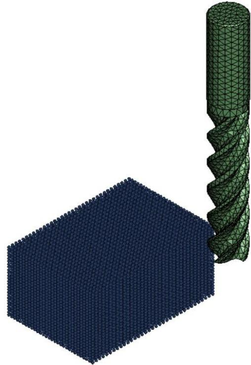
Fig. 8. Milling test simulation on isometric view
