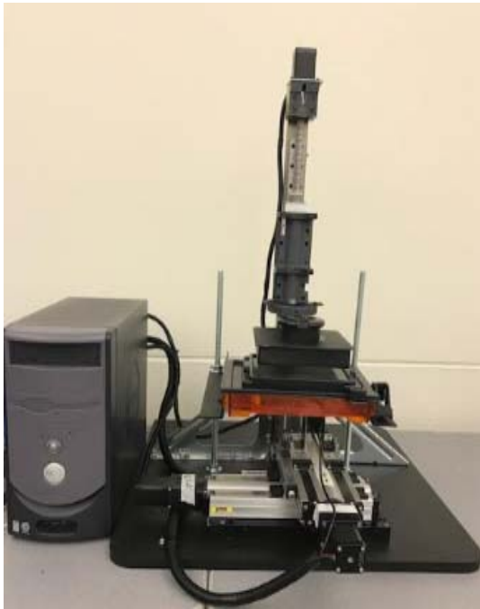
Fig. 10. Completed SLA printer
