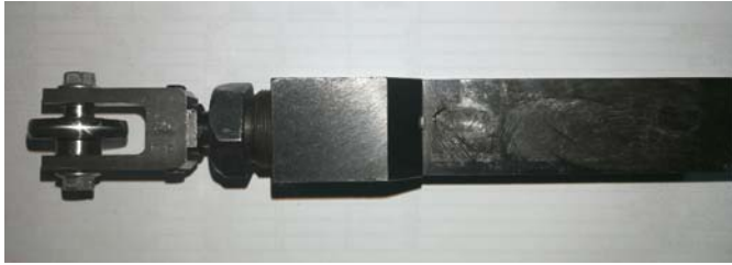
Fig. 5. A specially designed deep rolling device with a toroidal roller
