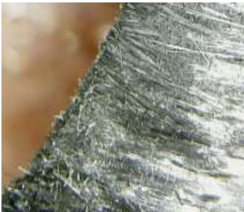
Fig. 5. The quality of the hole processing \varnothing 3.0 mm in the material VKU-25
