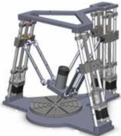
Fig. 2. 3D-model of the machine of frame configuration with MPS
