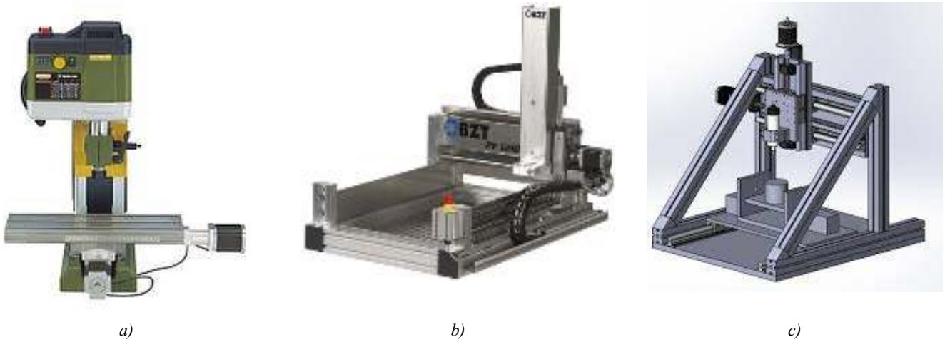
Fig. 1. Small-sized milling machines: a console type (a), traveling gantry machine, (b) machine with a moving table (c)
