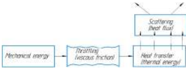
Fig. 2. Scheme of physical processes diagram of a hydraulic damper
