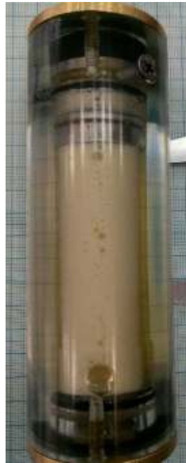
Fig. 7. The process of the origin of foaming and cavitation in the working chamber of the damper operating mode throttle: ( t = 20^{\circ}\text{C} )
