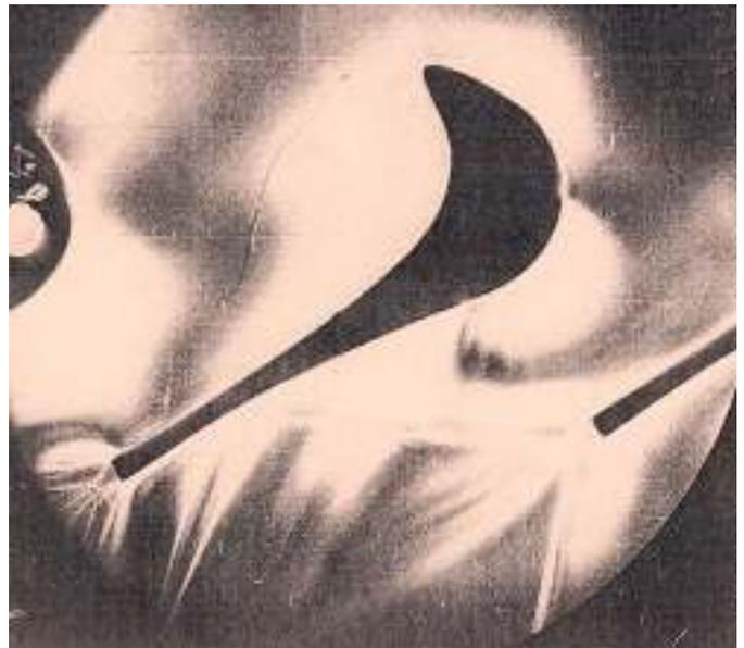
Fig. 4. The fluid flows in back concave blade profile on the aerodynamic stand at  $M = 1.32$
