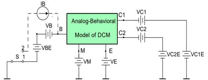
Fig. 1. Simulation setting for studying of static magnetolectric characteristics of a dual-collector magnetotransistor using analog-behavioral model
