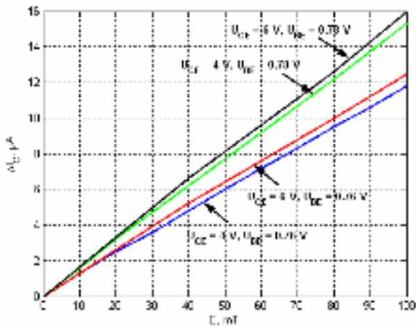
Fig. 3. Tesla-ampere characteristics  $\Delta I_C = f(B)$  at  $U_{BE} = 0.76V; 0.78V$  and  $U_{CE} = 4V; 6V$
