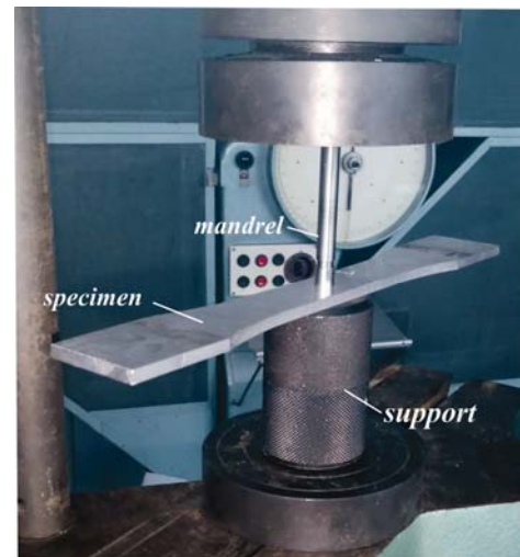
Fig. 4. Solid mandrel cold working process
