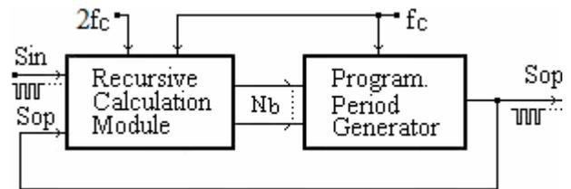
Fig. 7. The functional scheme of FLL.
