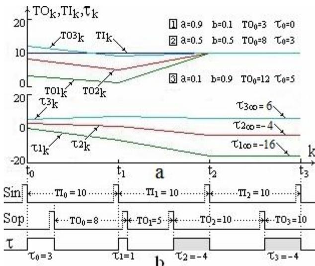
Fig. 4 a. Transition states of FLL for the step input and different system parameters, b. Real time presentation of Sin, Sop and  $\tau_k$  for the simulated case Nr 2.
