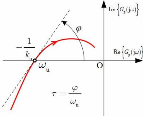
Fig. 1. Illustration of tangent rule
