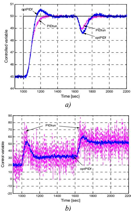
Fig. 3. Controllers in the loop with the model  $G_m(s)$  of the laboratory thermal process, a  $-20\%$  change of the control signal is inserted at time  $t=1600\text{s}$ . Comparison of the  $PID_{tun}$  and the proposed  $optPID_f$ , band-limited white noise  $nW(t)$  is added, with  $\text{PSD}=0.003$  and  $T_s=1$ .
