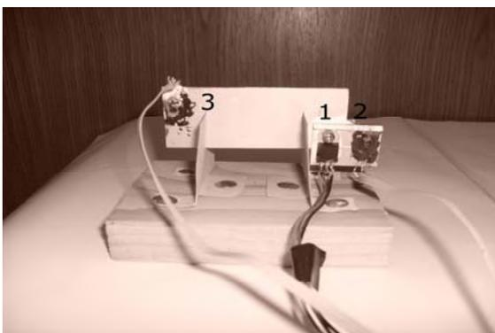
Fig. 2. Laboratory thermal plant with heater 1 at  $x=0$ . Temperature  $T(x,t)$  is distributed along the plate from  $x=0$  to  $x=L$ . The controlled variable  $y(t)=T(L,t)$  is measured by the sensor 3. Temperature sensor 2 at  $x=0$  is used in the safety device, to prevent overheating when  $T(0,t) \geq 70^\circ\text{C}$ .
