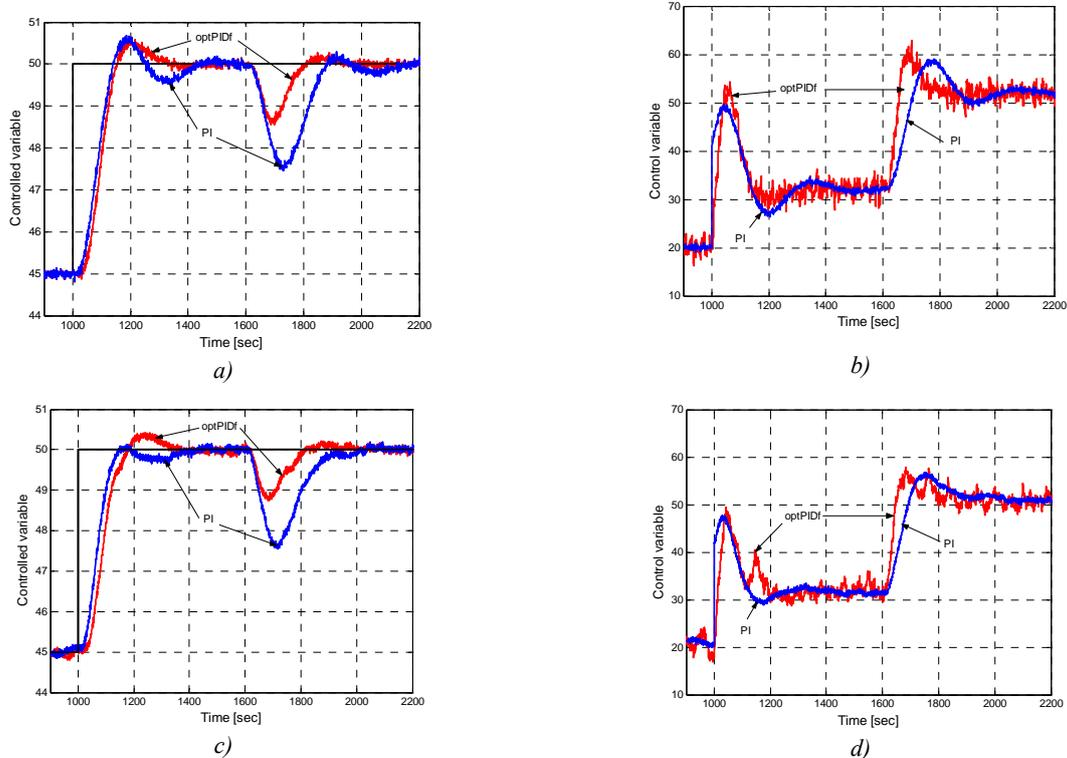
Fig. 4. The laboratory thermal process: a)-b) Simulation results, the evaluated PI and proposed optPIDf controller in the loop with the model  $G_m(s)$ , band-limited white noise  $nw(t)$  is added, with  $PSD=0.003$  and  $T_s=1$ ; c)-d) Real plant with the evaluated PI and proposed optPIDf controller. A -20% change of the control signal is inserted at time  $t=1600s$
