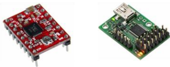
Fig. 5. Step motor driver cards
