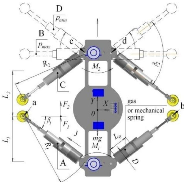
Fig.3. Scheme of the mobile robot (plan view)
