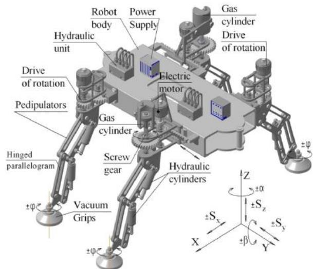
Fig. 2. Walking mobile robot with energy accumulators
