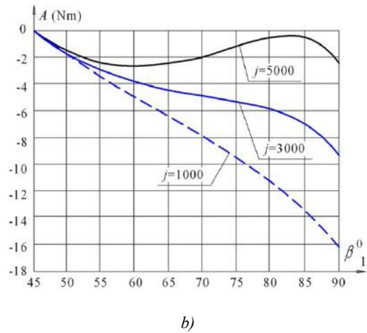
Fig.4. The effect of the rigidity  $j$  (N / m) of the elastic element on the speed (a) and the work performed by this element (b) in the second stage  $\beta_1 > 45^\circ$ , when the robot moves under the action of kinetic energy.
