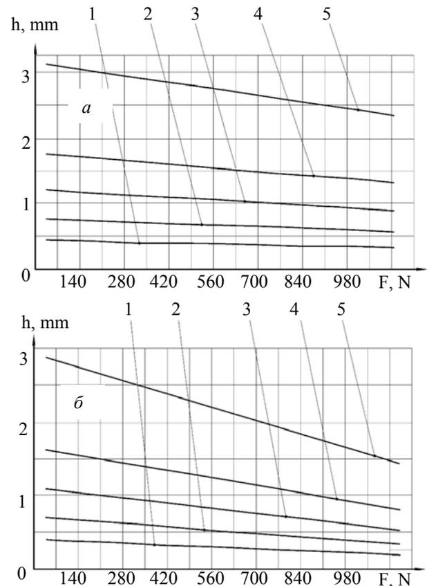
Figure 5. Correcting diagrams of displacement step recalculation: dispenser length 2,5 m (a) and 5,0 m (b) and diameters 1 – 6 mm, 2 – 8 mm, 3 – 10 mm, 4 – 12 mm, 5 – 16 mm
