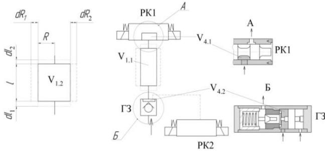
Fig. 2. Calculating diagram of dispenser:  $V_{11}$  – dosing chamber, A, Б – shut-off devices, PK1 – main directional valve, PK2 – feeding valve of the dosing chamber,  $V_{41}$  та  $V_{42}$  – valves inner volume
