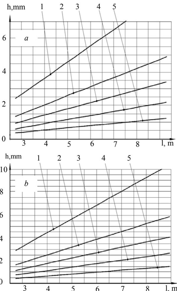
Figure 4. Definition of dispenser parameters by displacement step  $h$  without load at pressure 50 bar (a) and 60 bar (b): 1 – 16mm, 2 – 12mm, 3 – 10mm, 4 – 8mm, 5 – 6mm
