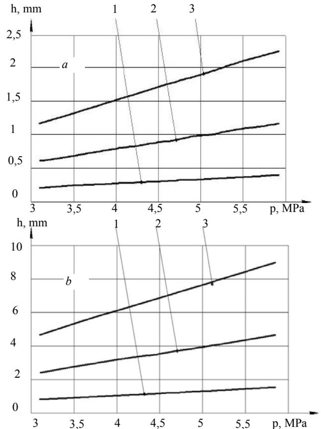
Figure 3. Piston displacement per pulse on pressure height: diameters 8 mm(a) and 12 mm (b); length: 1 – 2,5 m, 2 – 5 m, 3 – 7,5 m
