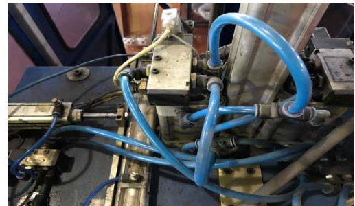
Fig. 3. Initial mechanism of the top plate of the clamp driven by pistons
