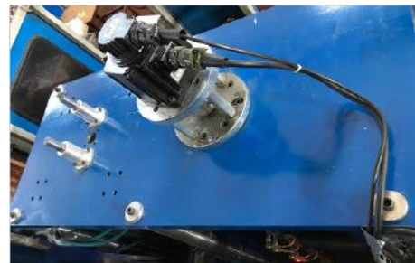
a) Servo motor in the assembled position
