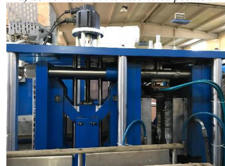
b) Clamp system (Open position)
