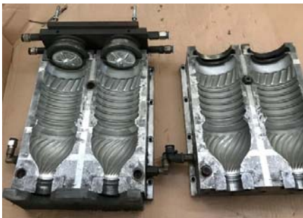
Fig. 2. A sample multi cavity mold type used in the experiments
