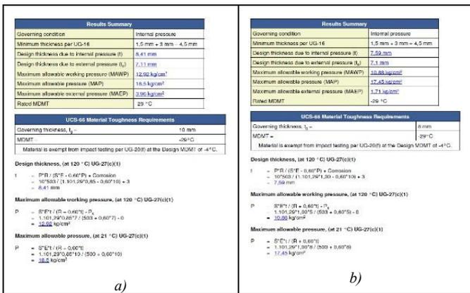
Fig.2. Thickness calculation summary screen of main body for SA-285 GRC
