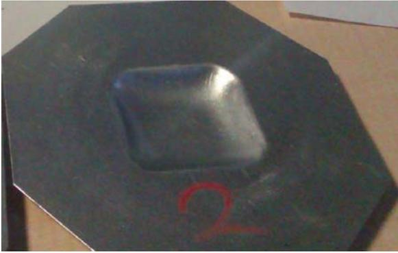
Fig. 14. Formed St12 specimen under 200bar pressure for second mould design
