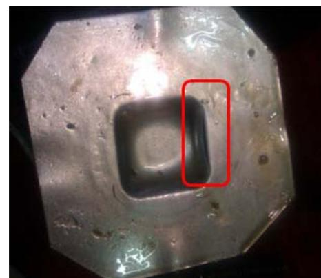
Fig. 7. Failed St12 specimen under 100bar pressure for first mould design
