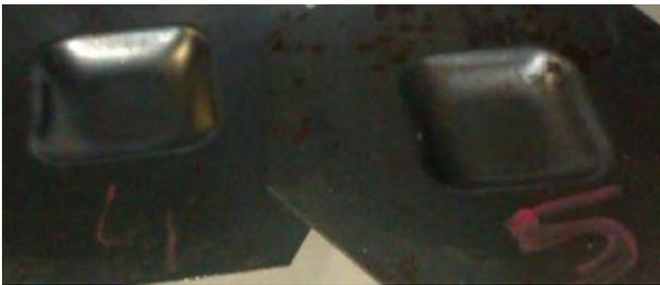
Fig. 17. Formed Sae 1006 specimen under 200bar pressure for second mould design
