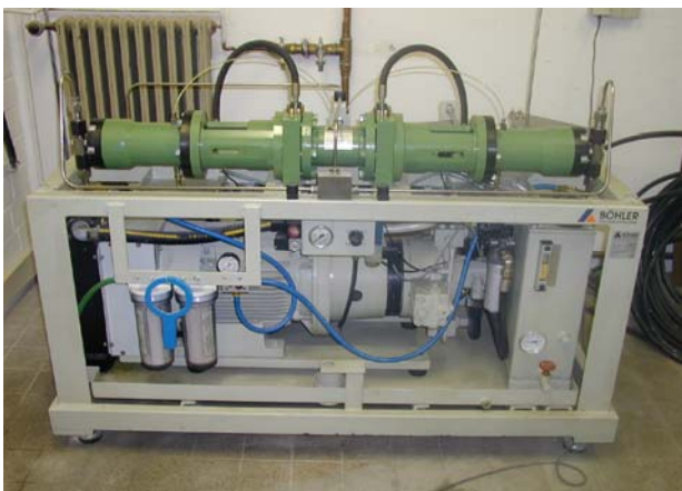
Fig. 1. Hyper pressure intensifier pump with a pressure of 900 MPa
