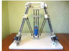
d) - machine-tool triglide with pyramidal frame layout and universal control system controller [4, 7]
