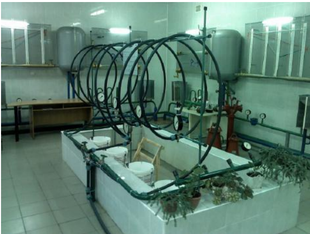
Fig. 2. The working part of the stand, which allows simulating the flow of viscous and abnormally viscous liquids with a variable along the flow mass
