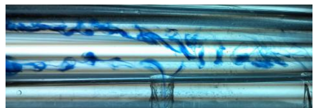
Fig. 6 The destabilization of the flow in the current behind the nozzle at Reynolds numbers Re>1500
