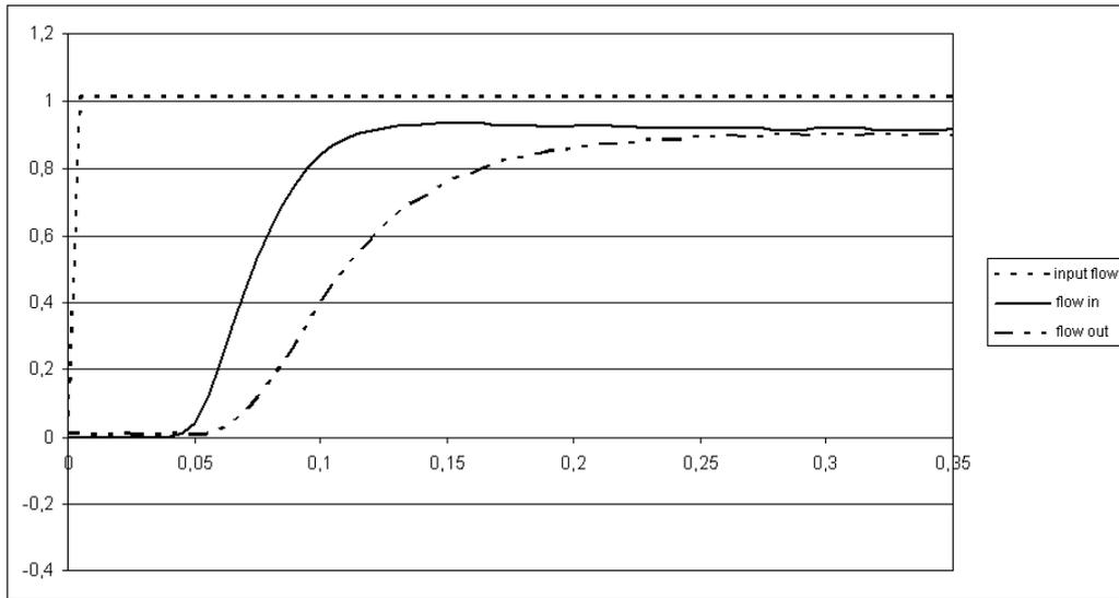
Fig. 2: Tube outlet flow for a constant flow input
