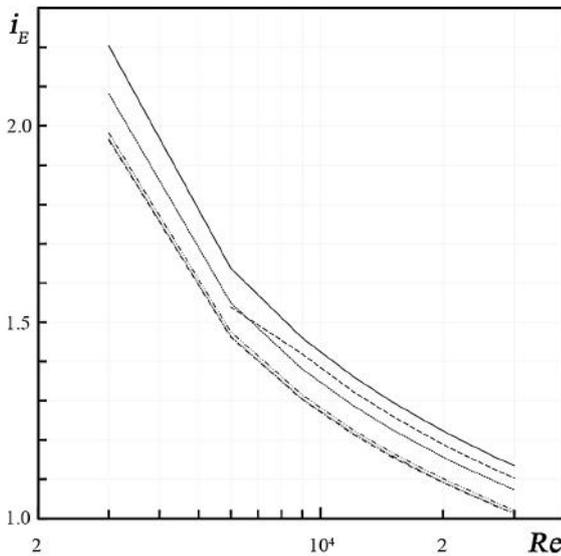
Fig.3. The variation of  $i_E$  with Reynolds number. Experimental results of García et al. [6].
