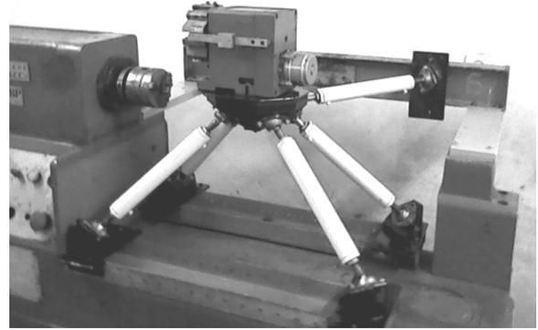
Fig. 2. The test bench for determining of the dynamic characteristics of the machine
