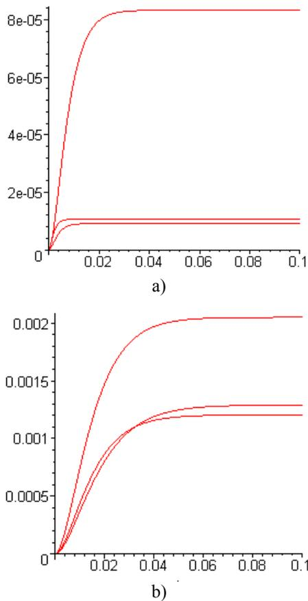
Fig. 3. The value of the end-effector realising and the time to start stable cutting process a: -the linear movement of the end-effector mass center (linear realise); b -the angular movement of the end-effector in the cutting process
